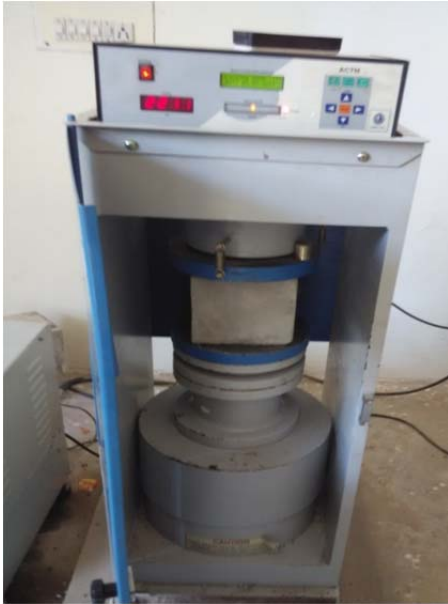
Fig. 3.2.1: Compressive Strength Testing Machine
