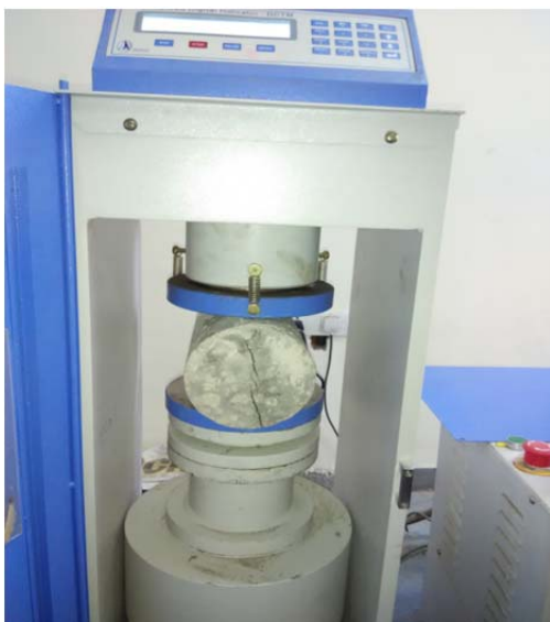
Fig. 3.2.2: Split Tensile Strength Test Machine
