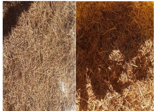
Fig. 2: Pictorial view of pine needles before and after grinder
