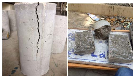
Fig. 3: Photograph indicating crack pattern specimen
