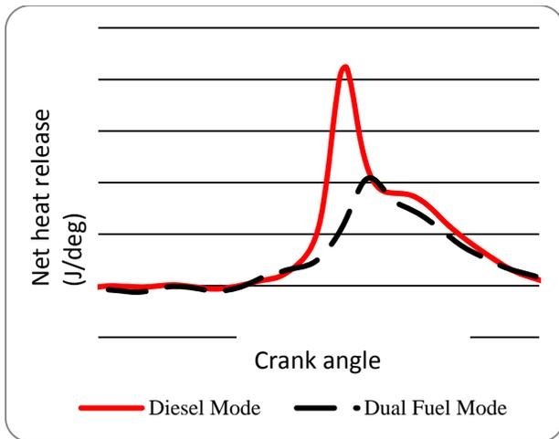
Fig. 3 Net heat release variations with respect to crank angle.
