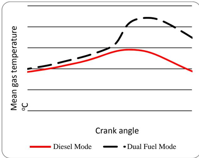
Fig. 2: Variations of mean gas temperature with crank angle.
