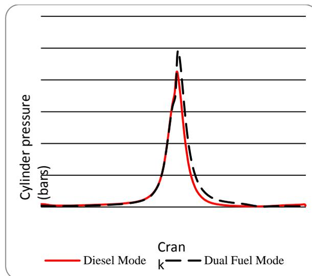
Fig. 1 Variation of cylinder pressure with crank angle.
